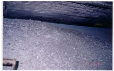
1,700 to 2,000 lbs. of scale removed
