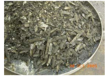
Scale collected from the evaporative condenser
