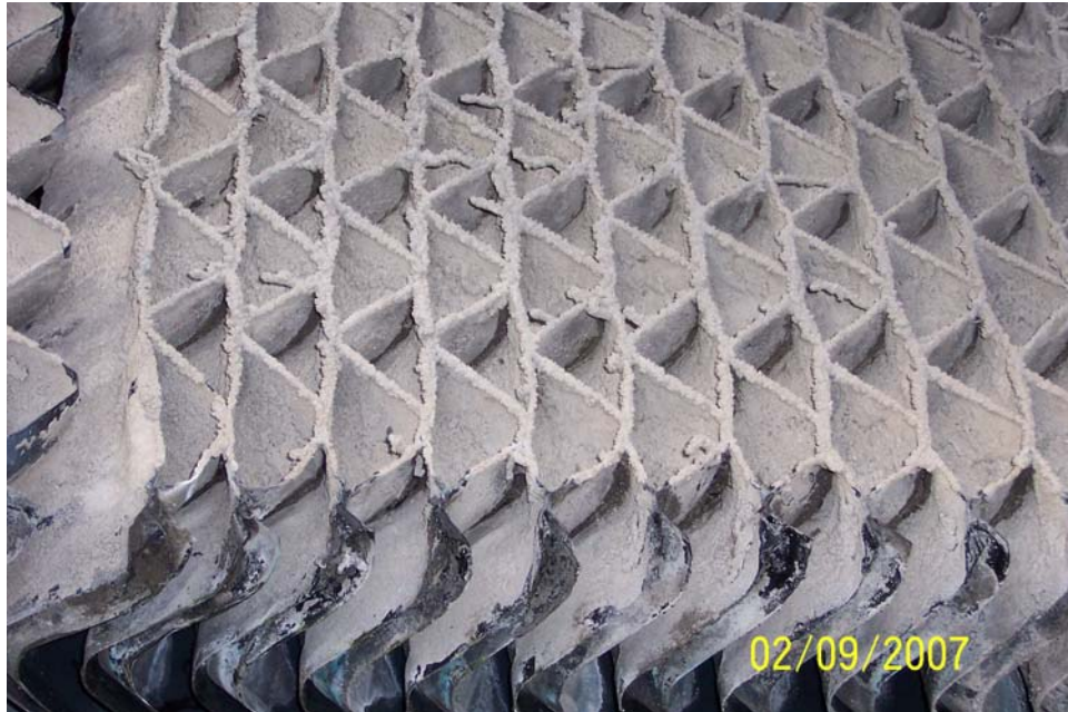
Top-side drift screens on day 1 of the evaluation, encrusted with scale.
